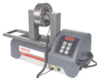
Hanging, with yoke through the workpiece
