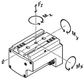
The indicated permissible forces and torques apply to a single gripper jaw. They include the lever arm, additional applied loads due to the workpiece or external gripper fingers and acceleration forces occurring during movement.
