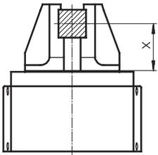
Gripping force  $F_h$  per gripper jaw
